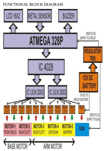
The block diagram explains the hardware components of the unmanned tanker robot. We have and LCD of the 16 by 2 dimensions which is fed the output by the main Micro controller i.e. ATMEGA 328P. The buzzer also receives the output from this micro controller. ATMEGA 328P feeds the output to the IC 4028 which provides a divided output to both IC ULN 2003.Metal sensor also feeds the output to ATMEGA 328P.
